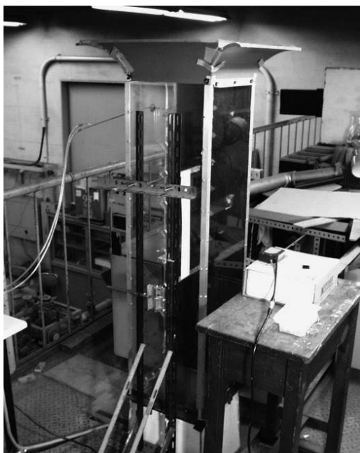
Fig.2 Test section of the vertical wind tunnel
